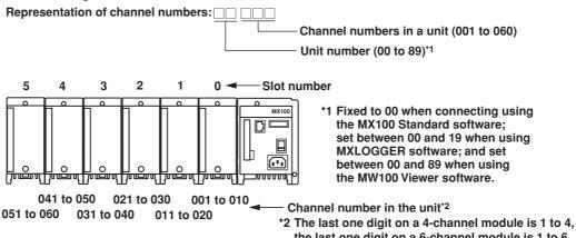
the last one digit on a 6-channel module is 1 to 6, the last one digit on a 8-channel module is 1 to 8.
