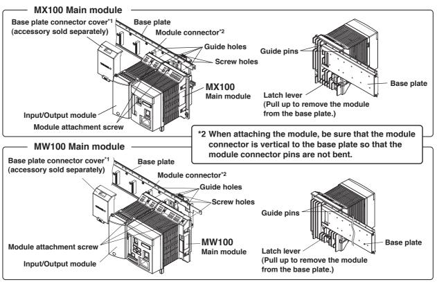
\*1 Can be attached by hooking the top section of the cover to the top edge of the base plate and pressing down on the lower section of the cover
